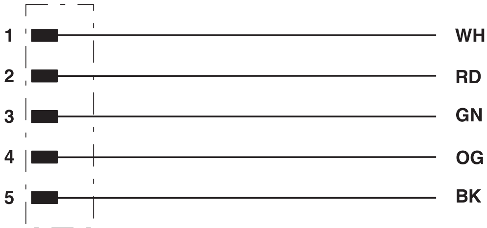
Contact assignment of 7/8" plug
