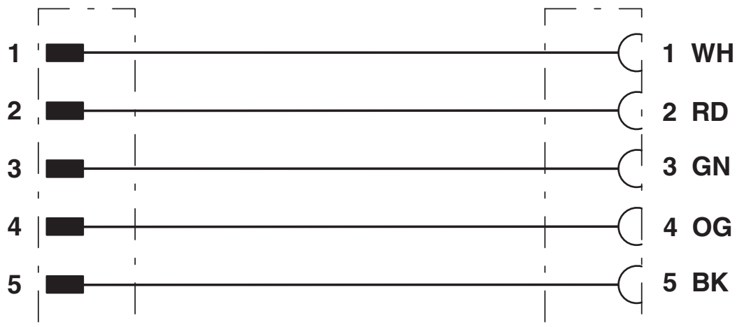
Contact assignment of 7/8" plugs/sockets
