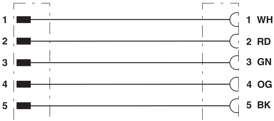
Contact assignment of 7/8" plugs/sockets
