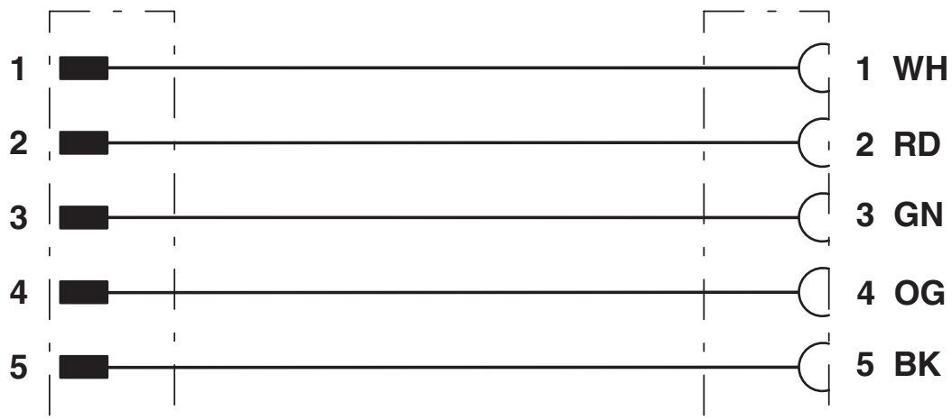
Contact assignment of 7/8" plugs/sockets
