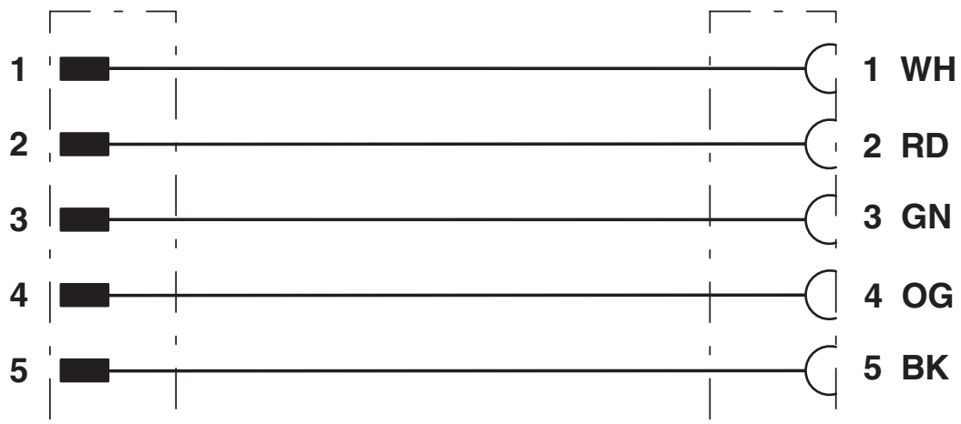
Contact assignment of 7/8" plugs/sockets
