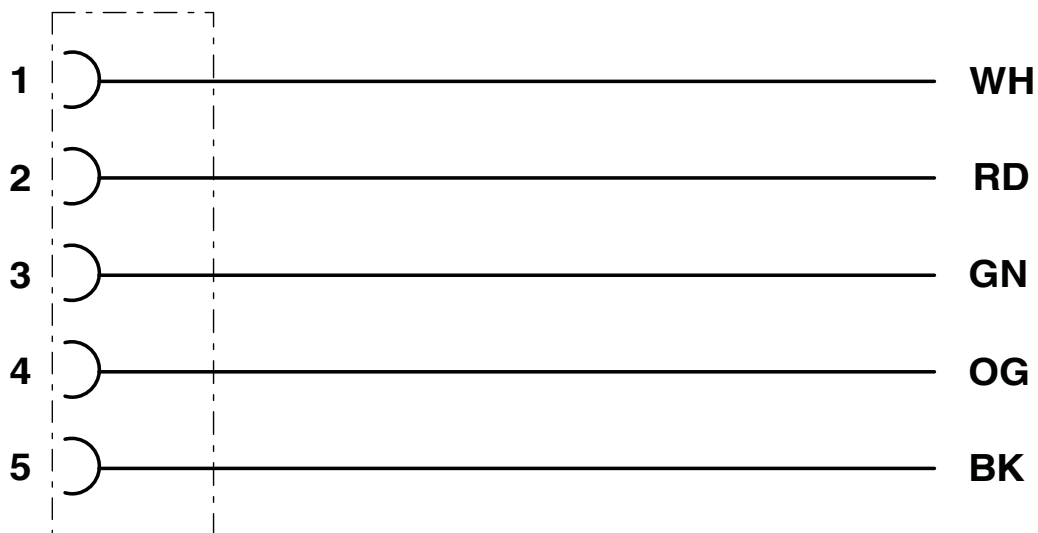
Contact assignment of 7/8" socket
