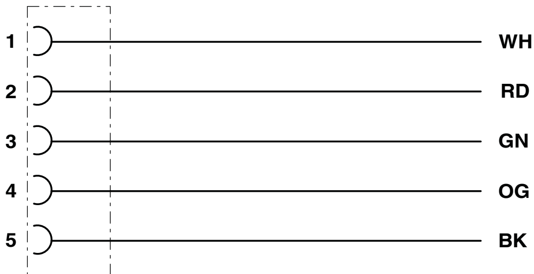
Contact assignment of 7/8" socket
