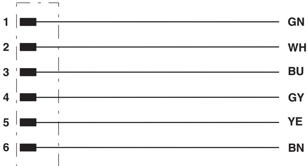
Contact assignment of 7/8" plug
