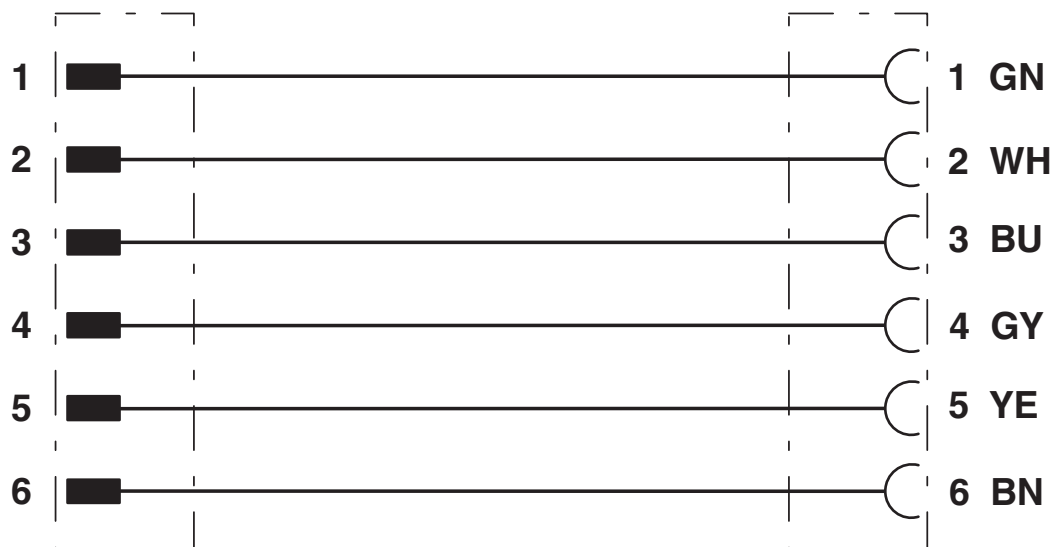
Contact assignment of 7/8" plugs/sockets
