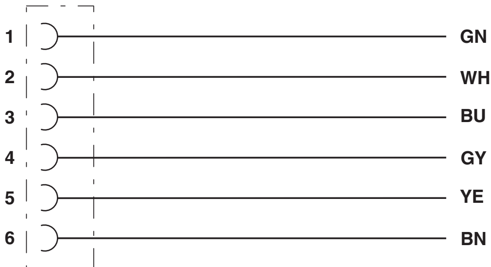
Contact assignment of 7/8" socket
