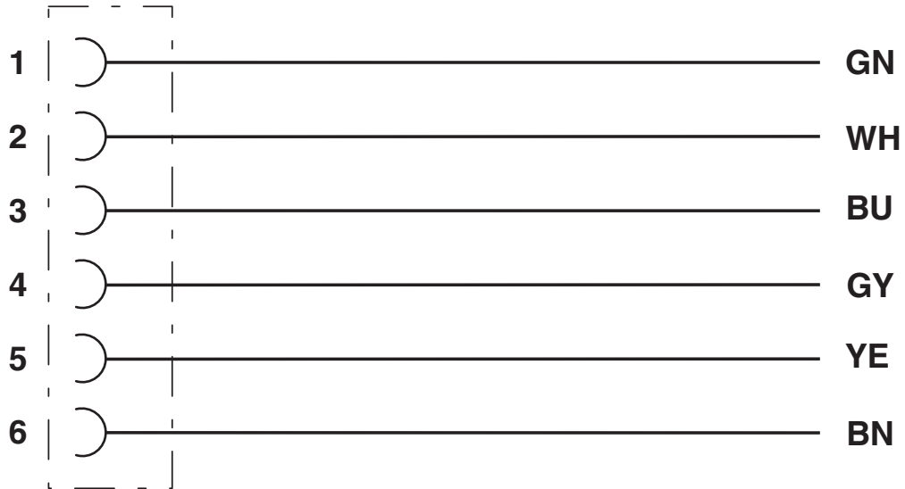
Contact assignment of 7/8" socket
