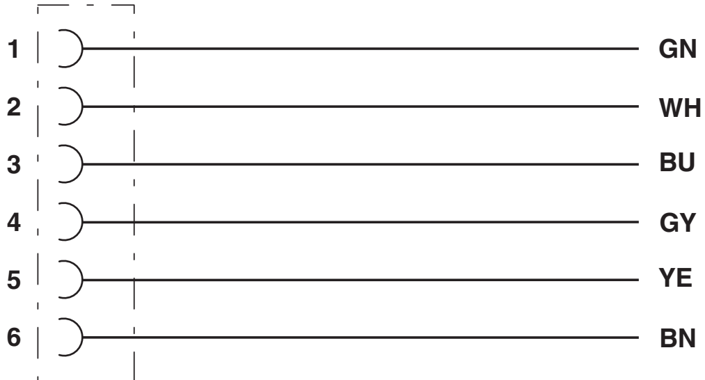
Contact assignment of 7/8" socket
