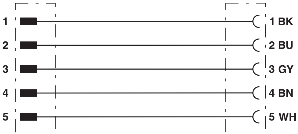
Contact assignment of 7/8" plugs/sockets
