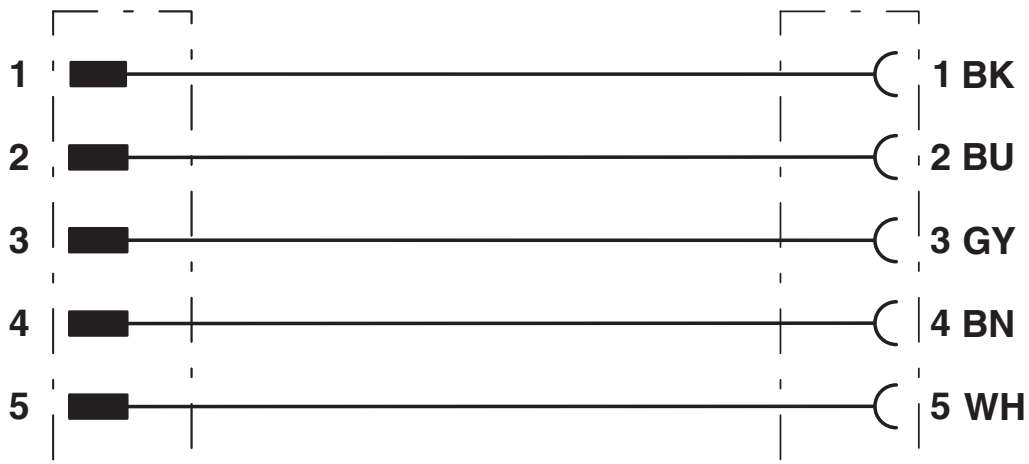
Contact assignment of 7/8" plugs/sockets
