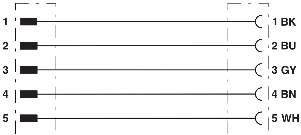
Contact assignment of 7/8" plugs/sockets
