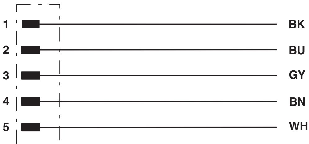
Contact assignment of 7/8" plug
