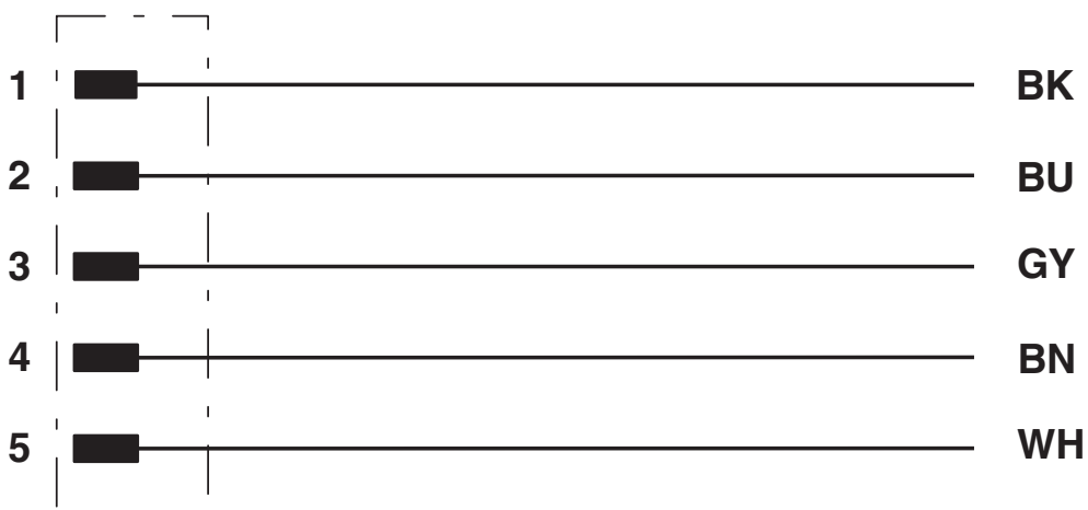
Contact assignment of 7/8" plug
