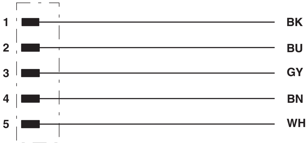
Contact assignment of 7/8" plug
