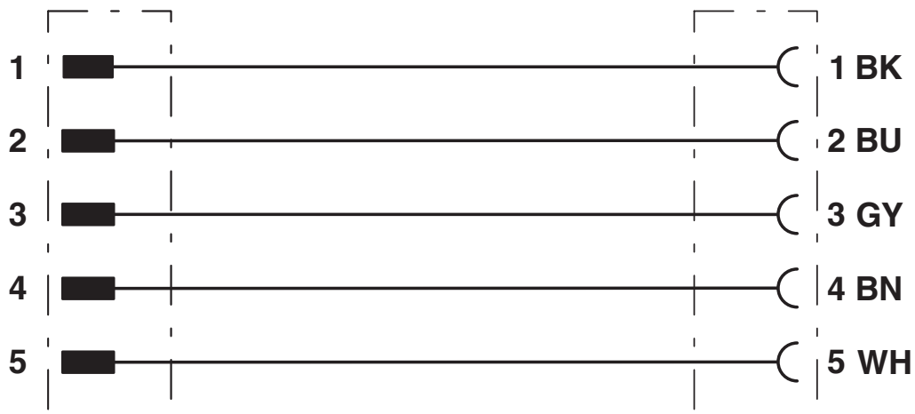
Contact assignment of 7/8" plugs/sockets
