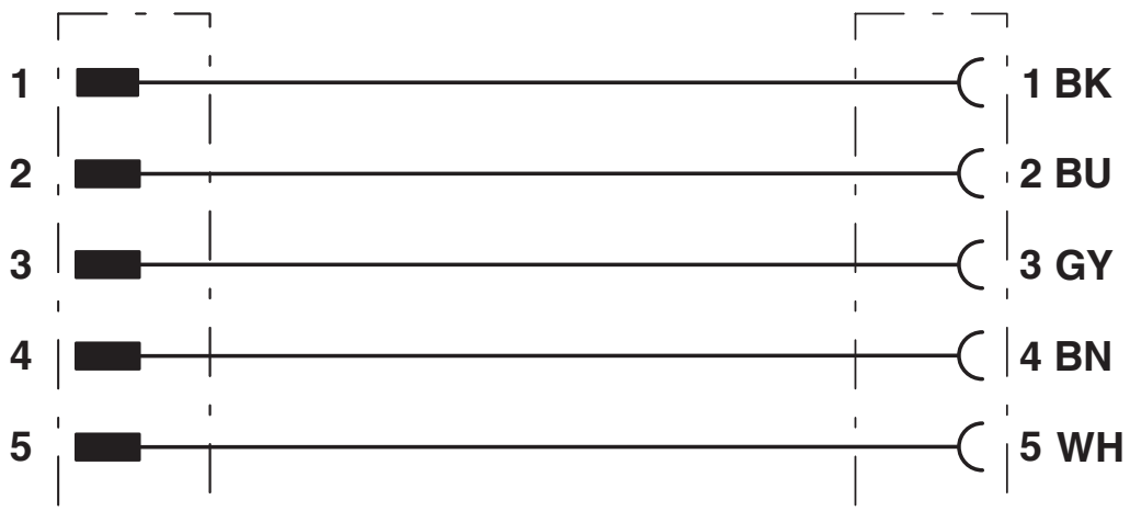
Contact assignment of 7/8" plugs/sockets
