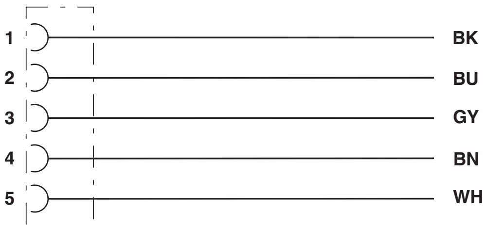
Contact assignment of 7/8" socket
