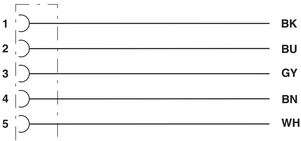
Contact assignment of 7/8" socket
