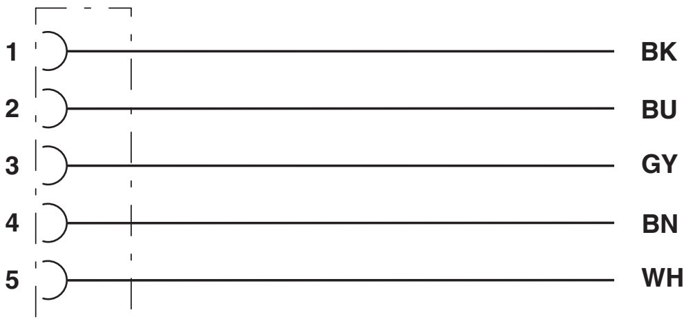
Contact assignment of 7/8" socket
