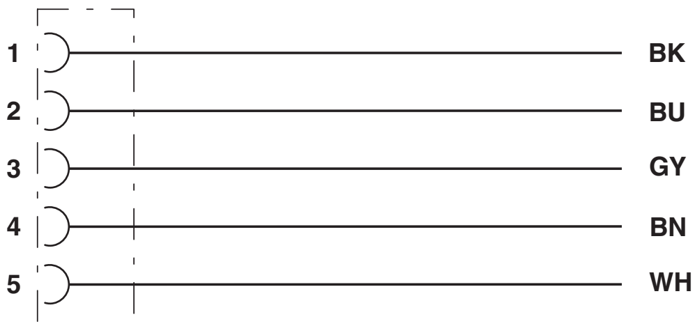
Contact assignment of 7/8" socket
