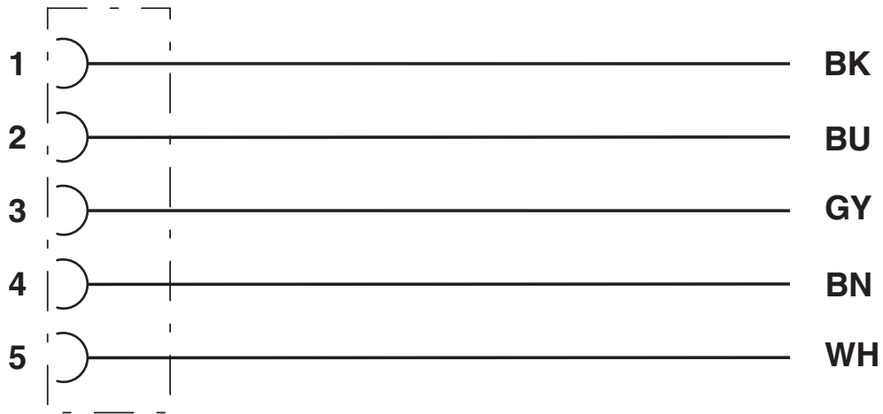
Contact assignment of 7/8" socket
