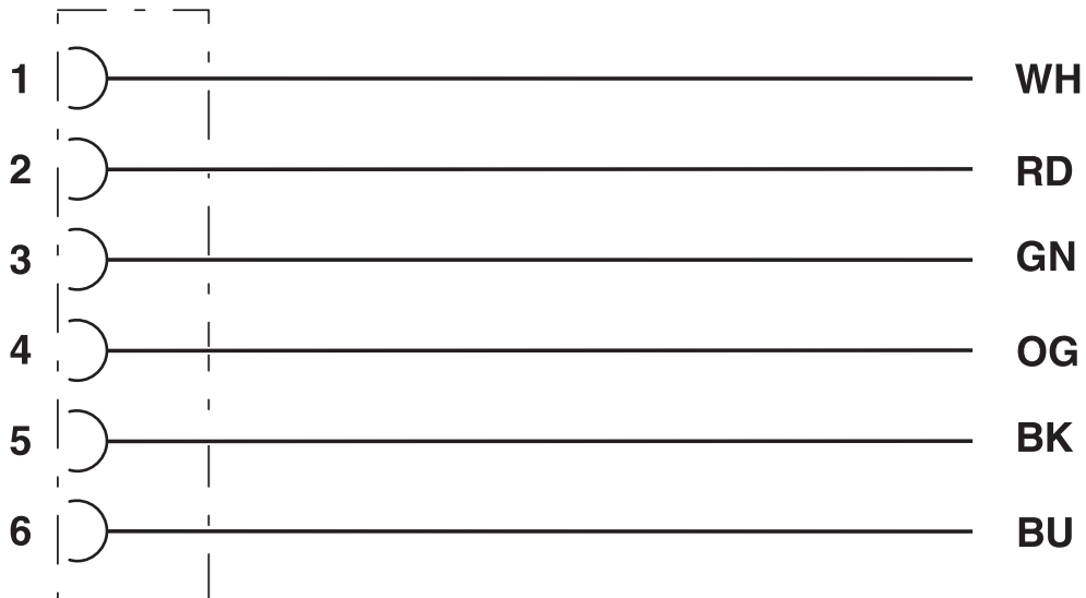
Contact assignment of 7/8" socket
