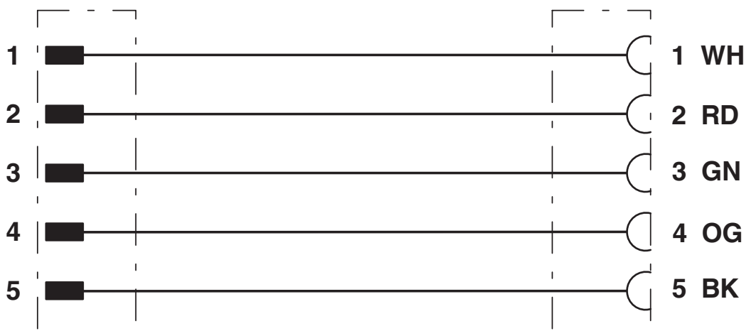
Contact assignment of 7/8" plug
