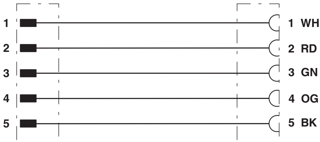
Contact assignment of 7/8" plugs/sockets
