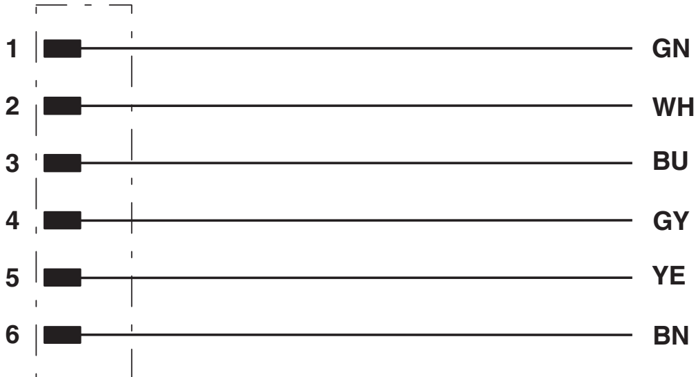
Contact assignment of 7/8" plug
