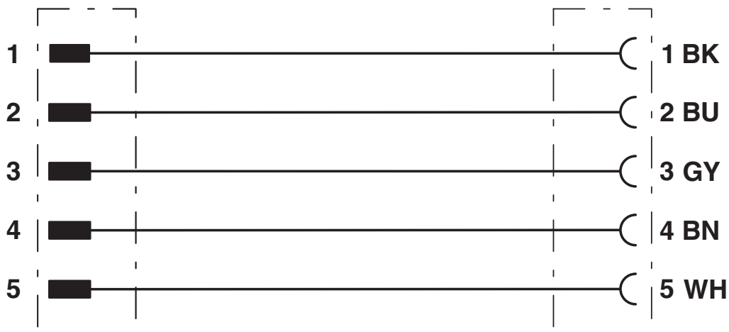
Contact assignment of 7/8" plugs/sockets
