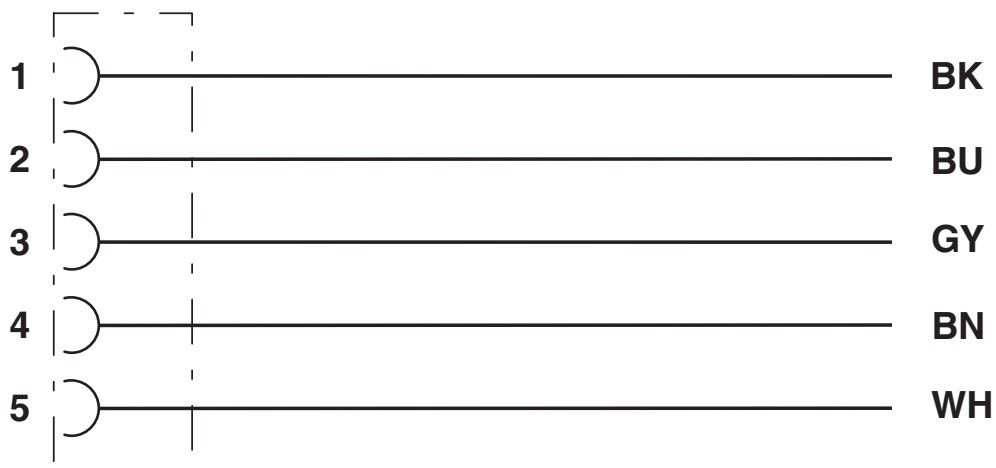
Contact assignment of 7/8" socket
