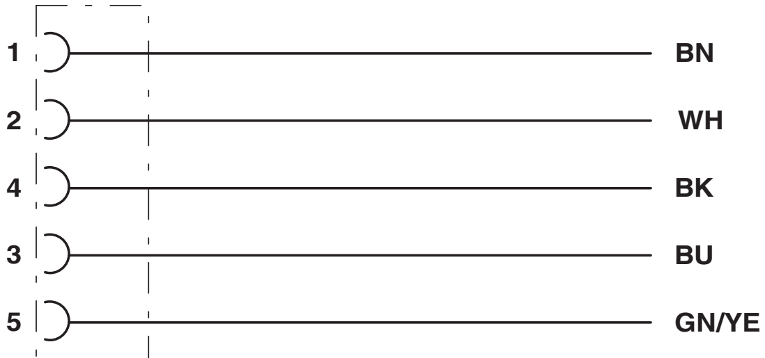
Contact assignment of the M12 sockets
