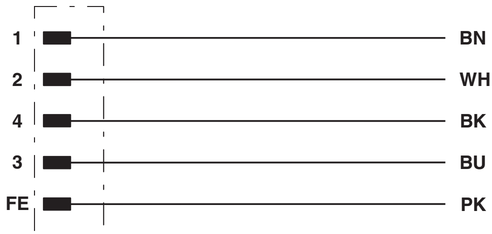
Contact assignment of the M12 plug
