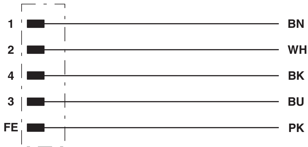
Contact assignment of the M12 plug
