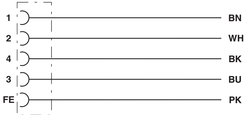
Contact assignment of the M12 socket
