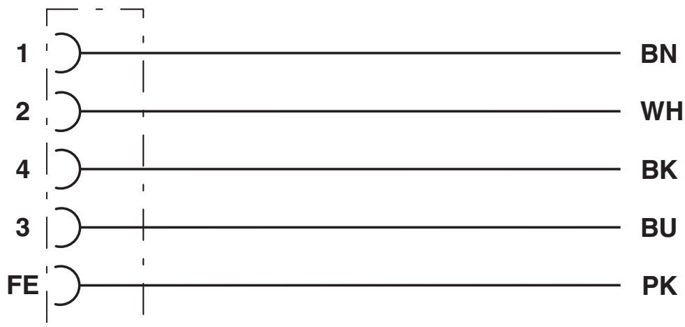
Contact assignment of the M12 socket
