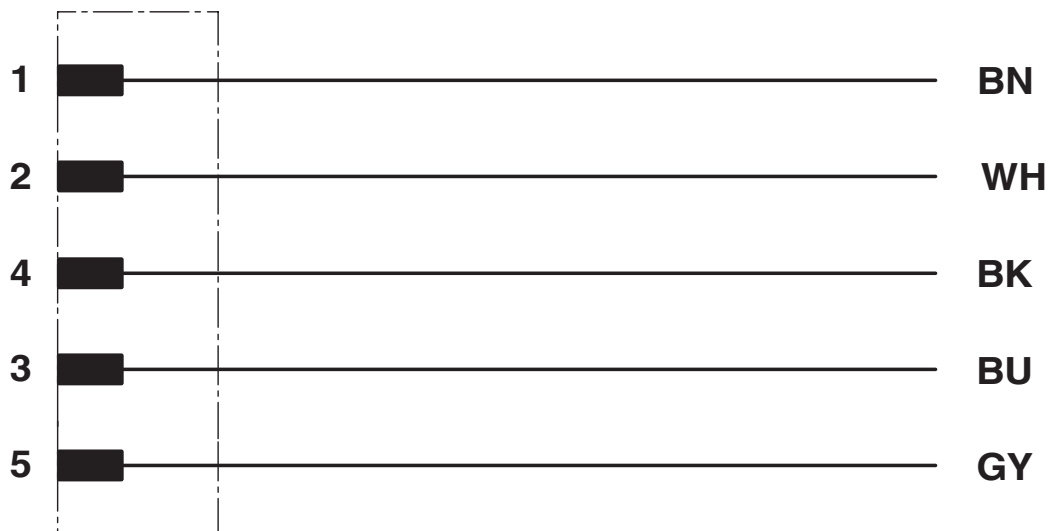
Contact assignment of the M12 plug
