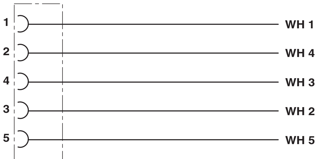
Contact assignment of the M12 socket
