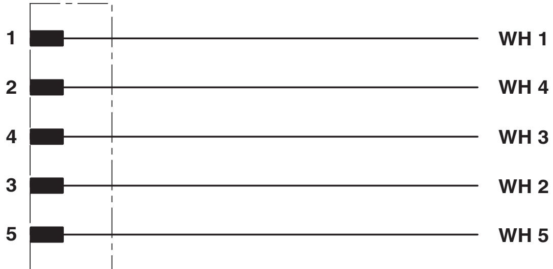
Contact assignment of the M12 plug
