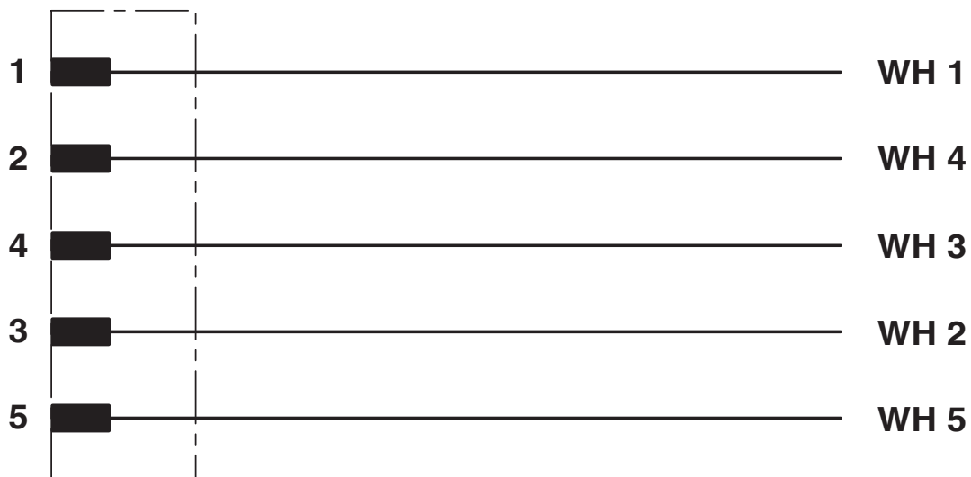
Contact assignment of the M12 plug
