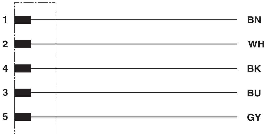
Contact assignment of the M12 plug
