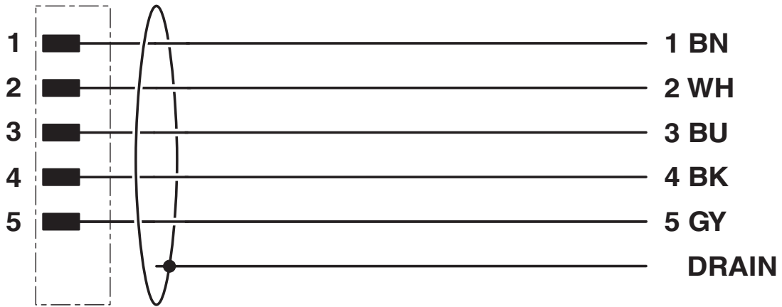
Contact assignment of the M12 plug and the M12 socket
