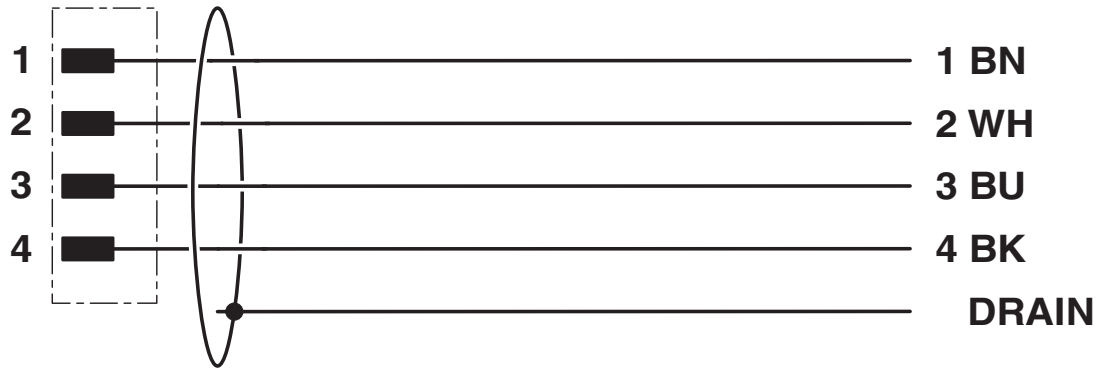
Contact assignment of M8 plugs/sockets
