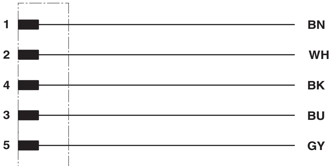
Contact assignment of the M12 connector
