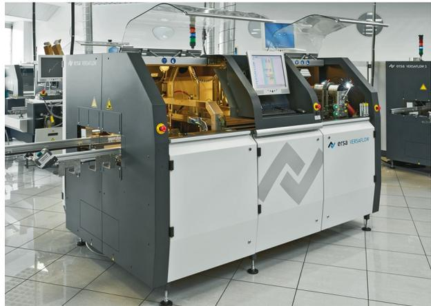
The PSR-MXF multifunctional safety relays are used in the Versa-Flow selective soldering system
