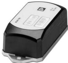
WLAN-Access-Point, client con due antenne interne (MIMO) per montaggio a vite, IP54, WLAN 802.11 a, b, g, n, frequenza: 2,4 GHz, 5 GHz (incl. canali DFS), collegamenti: COMBICON 9 ... 32 V DC, RJ45: per LAN, Web, http/https, Command Line Interface
