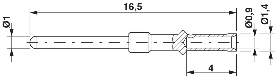
Crimpkontakt, Durchmesser: 1,0 mm
