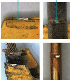
Figure 3 - Gas tightness in compliance with IEC 60512-6 – even after extreme weather simulations, the gas-tight electrical connection is verifiable using blank contact points, as shown in the examples of a pipe contact with a flexible cable (left) and with a massive cable with and without insulation (right) using blank contact zones.
