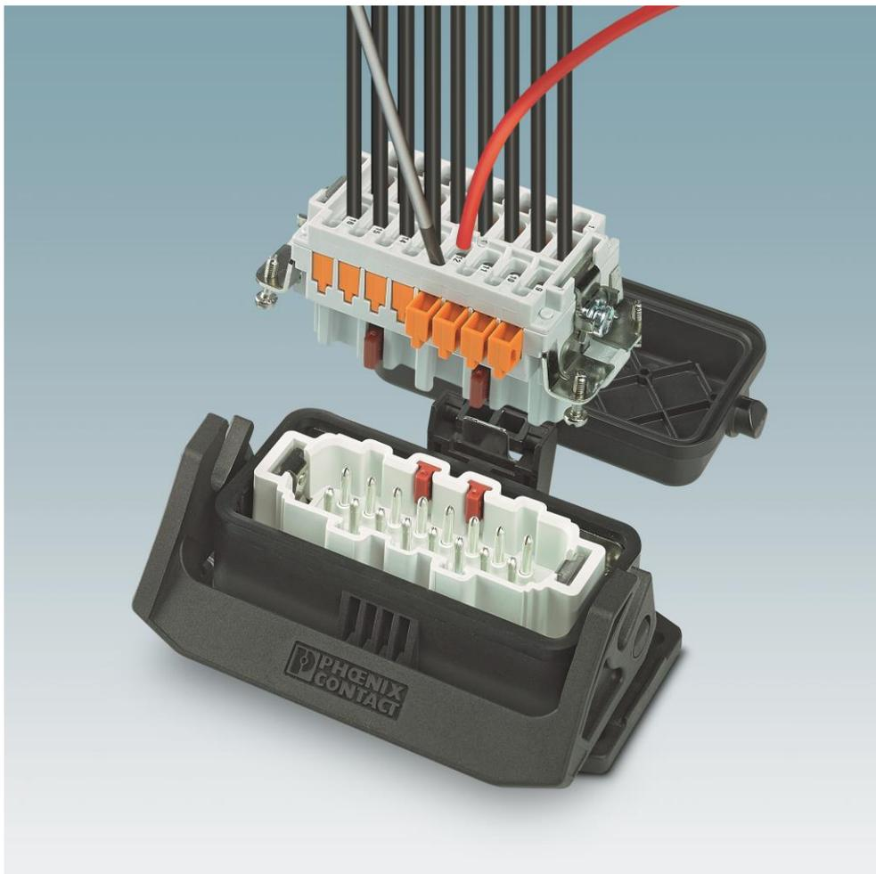
Figure 1, Lead Image - IDC connection for industrial plug-in connectors – this connection technology has been used for over a decade in a diameter range from 0.34 to 2.5 mm<sup>2</sup>.
