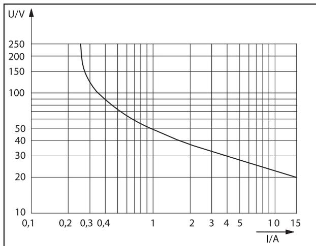
Figure 12 Example of a load limit curve (dependent on the type)
