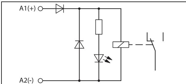
Figure 2 Block diagram of relay with DC input
