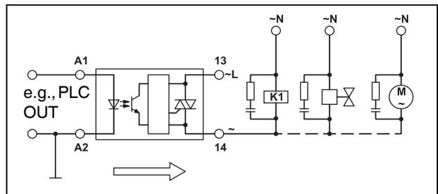
Figure 24 Example: Switching the contactor, solenoid valve or motor (AC load)
