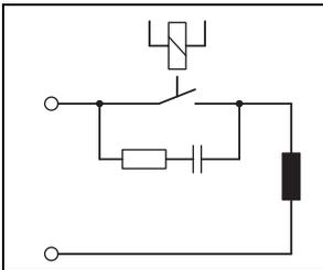
Figure 8 Contact protective circuit
