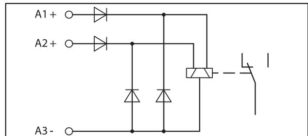
Figure 5 Block diagram of bistable relay, positive switching type
