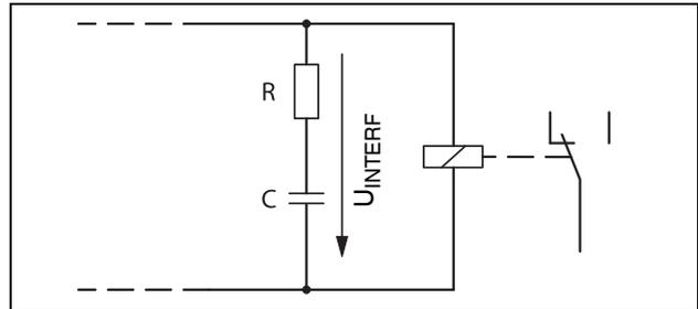
Figure 7 External RC interference suppression filter to prevent interference voltage coupling
