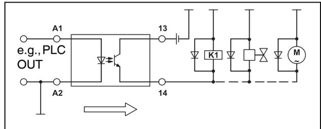
Figure 23 Example: Switching the contactor, solenoid valve or motor (DC load)
