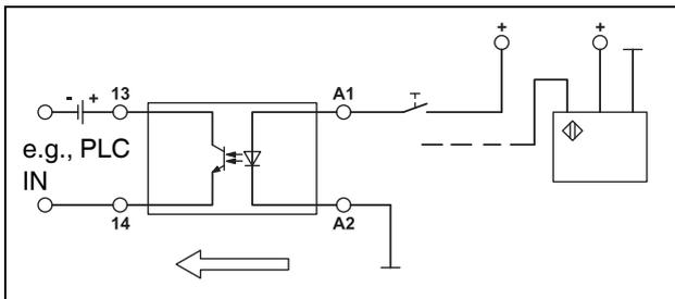
Figure 22 Example: Position indication with limit stop contact or initiator
