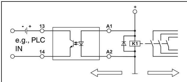
Figure 20 Example: Load contactor monitoring (DC contactor)
