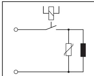
Figure 9 Inductive load protective circuit
