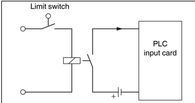
Figure 11 Application example: PLC input signal
