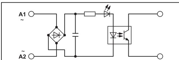
Figure 14 Block diagram AC input
