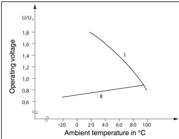
Figure 6 Sketch of a relay operating voltage characteristic
