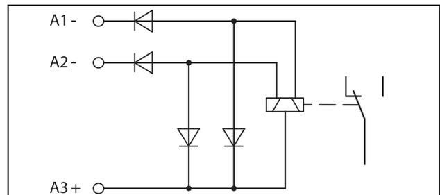
Figure 4 Block diagram of a bistable relay, negative switching type
