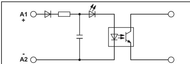
Figure 13 Block diagram DC input
