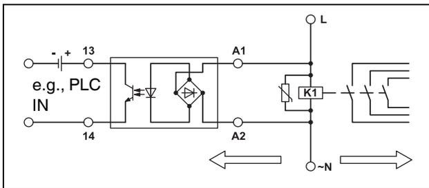
Figure 21 Example: Load contactor monitoring (AC contactor)
