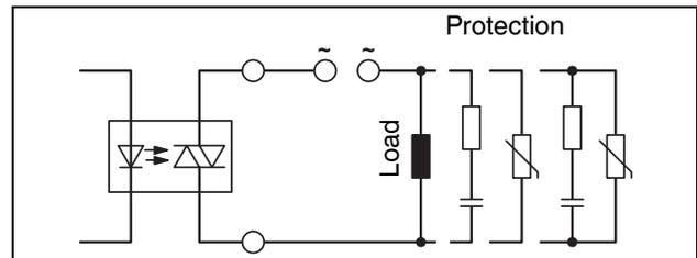
Figure 19 Protective circuit with AC voltage output
