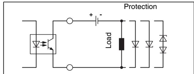
Figure 18 Protective circuit with DC voltage output
