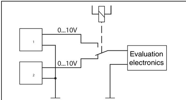
Figure 10 Application example: measurement point changeover
