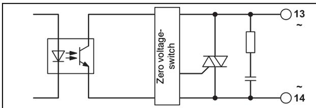
Figure 17 Basic circuit diagram of AC output
