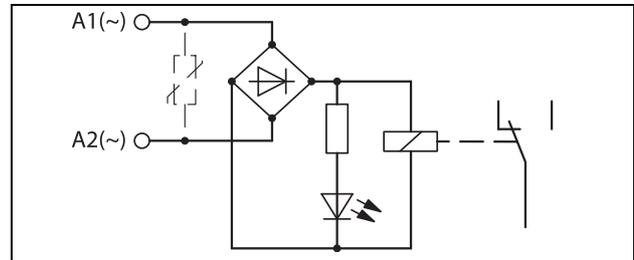
Figure 3 Block diagram of relay with AC/DC input
