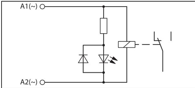
Figure 1 Block diagram of relay with AC input
