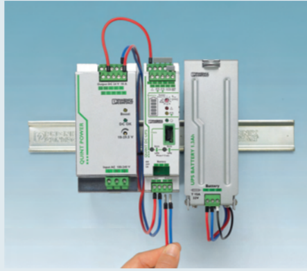
1.3. Connect the load to the UPS output.
