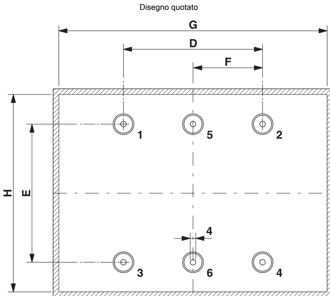
Misura D: 87,5 mm; E: 70,0 mm; G: 119,0 mm; H: 96,0 mm
