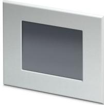
Pannello web, 17.8 cm / 7"-TFT display (Touch screen industriale resistivo), 800 x 480 pixel (WVGA), 65536 colori, Arm9™, 184 MHz, 2x USB Host 2.0, 1x Ethernet (10/100 MBit/s), RJ45, Windows® CE 5.0, MicroBrowser, senza sistema bus.
